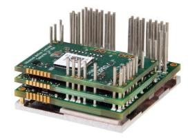
The **FE100-50-EM** is a FlexPro® series servo drive with IMPACT™ architecture.
