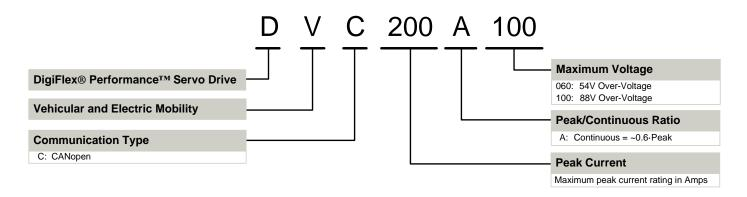
ADVANCED Motion Controls servo drives are available in many configurations. Note that not all possible part number combinations are offered as standard drives. All models listed in the selection tables of the website are readily available, standard product offerings.
