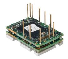
The **FE060-5-CM** is a FlexPro<sup>®</sup> series servo drive with IMPACT™ architecture.
