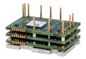
The **FE060-5-IPM** is a FlexPro<sup>®</sup> series servo drive with IMPACT™ architecture.
