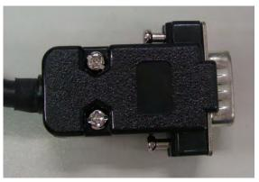
(3) Tighten the screws to complete the shielding.
