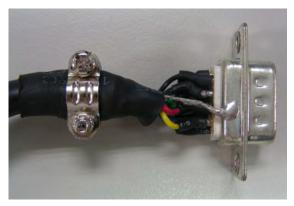
Solder the centre cores on the metal part of the connector adequately for good ground contact with the plate and shielding.
