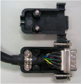
(2) Trim the ends of the cores and install the cores with shielding into the plastic case of the connector as shown in the figure.
