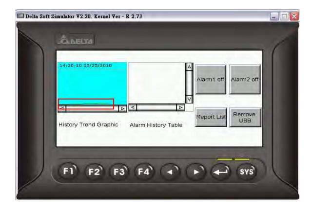
The user can press two Momentary button elements to enable and disable the alarms. The alarm data will be recorded in Alarm Data Table for user's reference.
